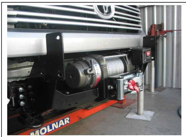
Figure 9 - Steel mount fitted.
